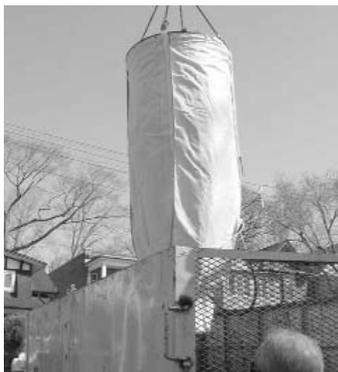
**A truck fitted with a hydraulic lifting arm is used to service the deep collection units.**
