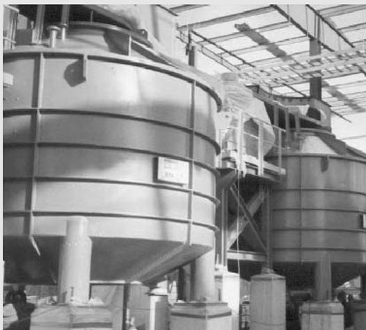
**Hydropulpers (above) are the first stage of the wet mesophilic anaerobic digestion technology, wetting, separating, then pulping the organic fraction. A rake-like unit (right) passes through the liquid to remove plastics and other floating light fraction material.**
